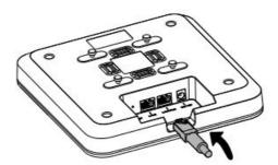
Connect the Ethernet cable to the LAN port
