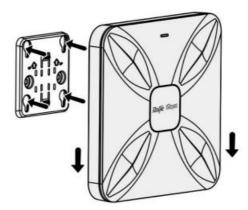
Align the square feet on the rear of the AP over the mounting holes on the bracket. Slide the AP into the holes until it clicks into place.
