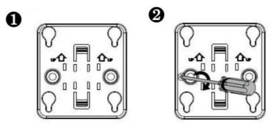
Attach the mounting bracket on the ceiling.
